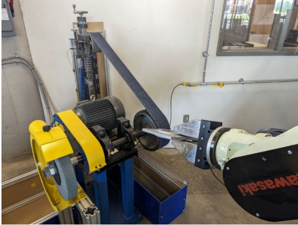
Figure 6. Parting line grinding is shown.
