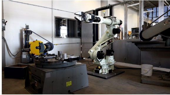
Figure 1. The casting finishing cell with material handling robot and related tools.
